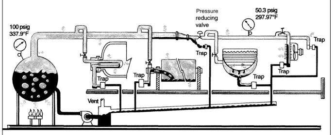
Heat radiation from the distribution system causes condensate to form. Steam traps, at natural low points or ahead of control valves, remove the condensate before it becomes a barrier to heat transfer. Hot condensate is returned through the traps to the boiler for reuse.
