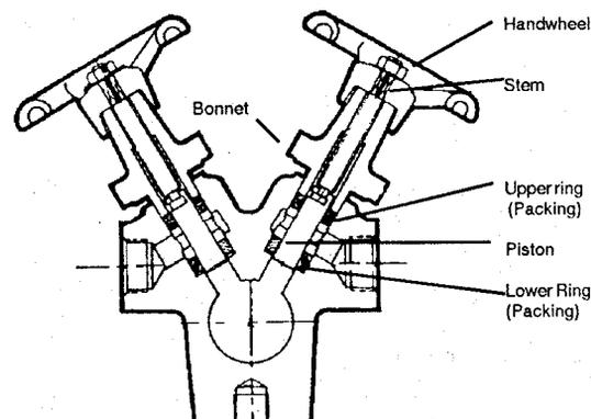
PTFE washer does soften as temperature rises. The softening helps the washer take the shape of the body and piston to assist sealing. The teflon helps lubricate the piston. Since the piston never clears the upper seals when open, the upper seals don't require metal reinforcement, and the softened PTFE is captured.
