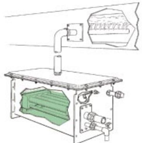
Electrode units are easily adaptable to different control signals and offer full modulated output. However, the need to boil the water means control will not compare with direct-injection units.
