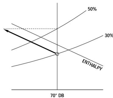
Water spray contains virtually none of the heat of vaporization required to increase the RH of the air to desired conditions. For this reason, water spray humidification is a virtually constant enthalpy process. However, as the psychrometric example illustrates, DB temperature changes as we increase RH from 30%-50%. The result of this loss of DB temperature is an increased heating load to maintain 70°F.
