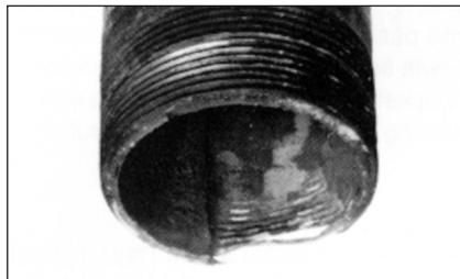
**Figure CG-9.** CO<sub>2</sub> gas combines with condensate allowed to cool below steam temperature to form carbonic acid, which corrodes pipes and heat transfer units. Note groove eaten away in the pipe illustrated.
