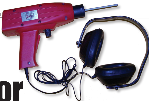
FIGURE 1. Traditionally, visual inspection has been the primary method of steam-trap testing. Manual inspections are aided by the use of temperature-monitoring and listening devices, such as the ultrasonic stethoscope shown here
