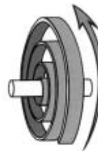
Bimetal principle has very little power
